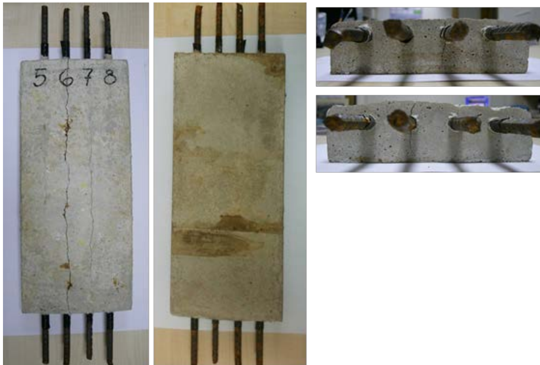
Fig. 1: short rolled bars embedded in concrete slabs.
