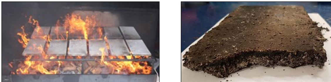
Fig. 2: Gypsum panels added with plastic waste during direct fire test (left) and after test (right)
